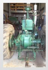
This tractor is started by using shot gun cartridges and is fully operational. Over the next few months it will be tidied up and prepared for the McFall Museum. Hearing the engine burst into life following the loud crack is quite something. Manufactured in Gainsborough in England in 1948 it was shipped to New Zealand and sold to the McCullough's of Temuka for 865 pounds.
